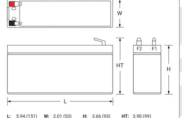
Tolerances are +/- 0.04 in. (+/- 1mm) and +/- 0.08 in. (+/- 2mm) for height dimensions. All data subject to change without notice
